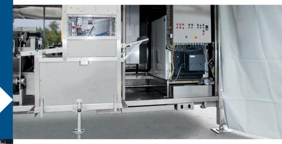
After a bag is placed in the locking device and the tap has been removed, the filling station is swung over the top of the bag and the start button is be pushed. The set amount is pushed into the bag with the filling pump.
