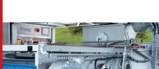
In order to adapt the machine to the different working conditions (fruit- and vegetable types), the belt speed and the crushing pressure can be changed by the user as needed. The assembly can be made with different hourly performance settings as desired, in order to accommodate individual production requirements.
