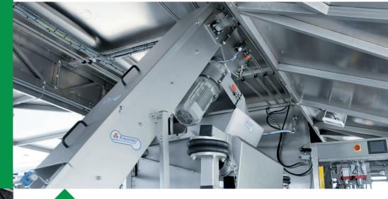
A food safe plastic conveyor belt with continuous speed setting transports the fruits upwards, where it gets cleaned again by water spray jets and is transferred into the directly attached crushing system. A highly efficient crushing system prepares the mash for a quick and simple pressing in a sophisticated process.
