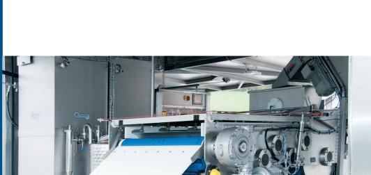
Our crushing machine combine innovative crushing technology and high performance with simple handling. The mash is passed through an adjustable dosing box, spread evenly on the sieve belt, and finally removed with a scraper.
