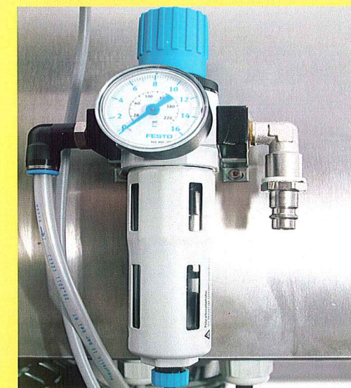
Pressurized air connection with pressure regulator
